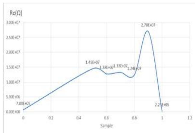
**Fig. 2**  $R_c$  (ohm) versus wt% of modified PuD-NaI
