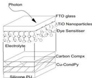
Fig. 1 DSSC cell diagram
