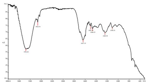
**Fig. 3** FTIR spectra of bio oil
