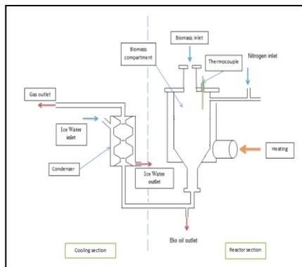
**Fig. 1** Schematic diagram of bio-oil produced via fast pyrolysi
