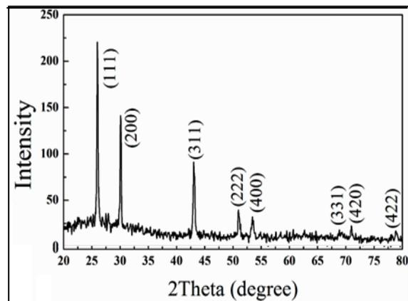
**Fig. 1** XRD pattern for the grown PbS thin films using 0.1M concentration of precursors.
