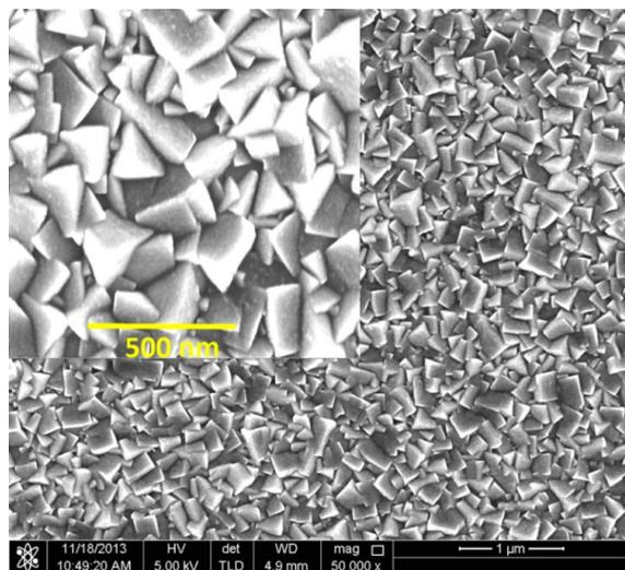
**Fig. 2** FESEM images for the grown PbS thin films prepared by the MA-CBD. The insets showed images with higher magnification.
