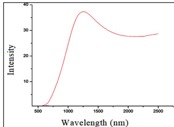
**Fig. 3** Transmission spectrum of nanostructured PbS thin films prepared by the MA-CBD.
